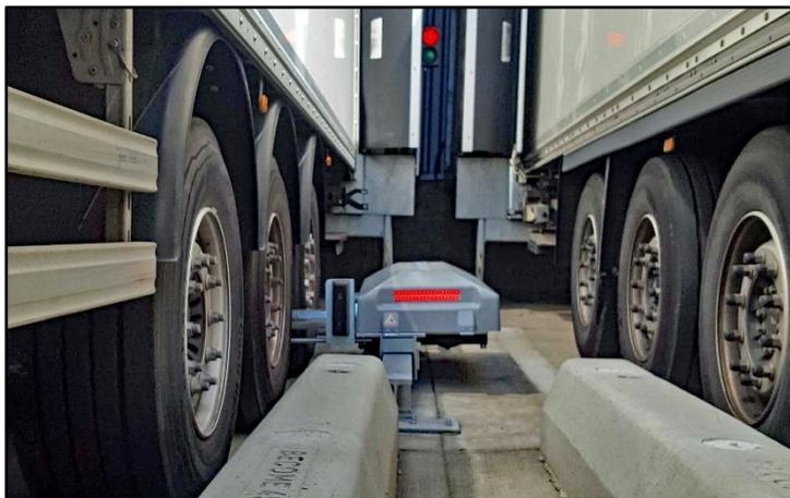
Autoblock is a machine designed to secure docking procedures and merchandise transshipment by immobilizing the truck's trailer while the loading / unloading procedure takes place.
