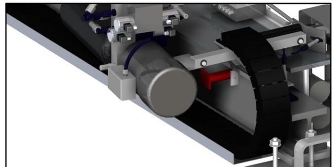
**Note:** The hydraulic unit must be moved (2 screws under the block) to be able to remove the rear axle.
