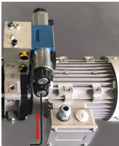
With the end of the Allen key, press the distributor's brass coloured nozzle and, at the same time, pull the wheel-stop's reinforcement leg to make the wheel-stop enter. The reinforcement leg must not be pressured on the truck's wheel. If the wheel-stop does not re-enter at all, do the same operation with the opposite coil.
